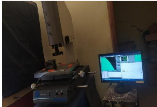
Figure 2 Exhaust Valve Drawing Prepared On Video Measuring Machine
