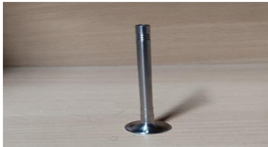
Figure 7 New 3D Metal printed exhaust valve
