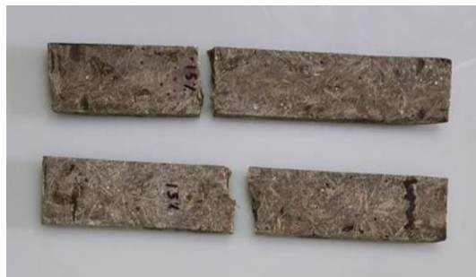
Figure 8. MB-3 (15% BFRC) After Tensile Test
