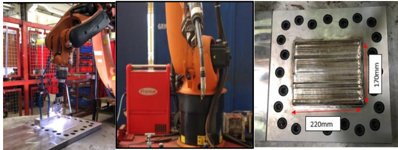
Figure 1. TIG and CMT setup with Fixture
