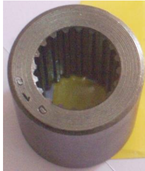
Figure 2 Splined Coupling typical size 35 mm diameter x 45 mm length
