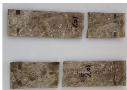
Figure 7: MB-2 (10% BFRC) After Tensile Test
