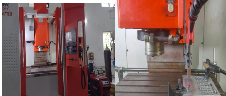
Figure 5. WAAM Experimental setup
