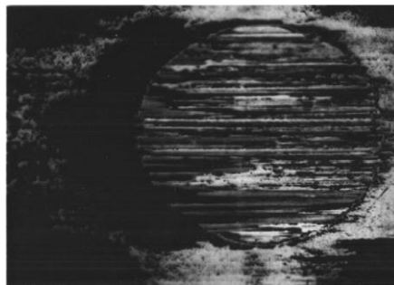
Figure 5 On a steel ball, a typical transfer layer generated during a sliding test in dry nitrogen (magnification: 50X).
