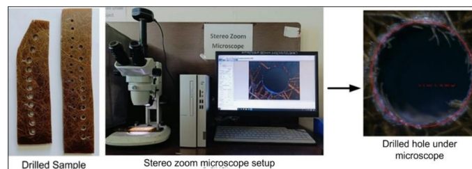
Figure 2 Microscopy assessment method of drilled hole
