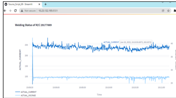
Figure 6: Real time weld monitoring
